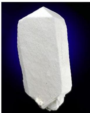
Bórax  $\text{Na}_2\text{B}_4\text{O}_7 \cdot 8\text{H}_2\text{O}$  - C2/c
